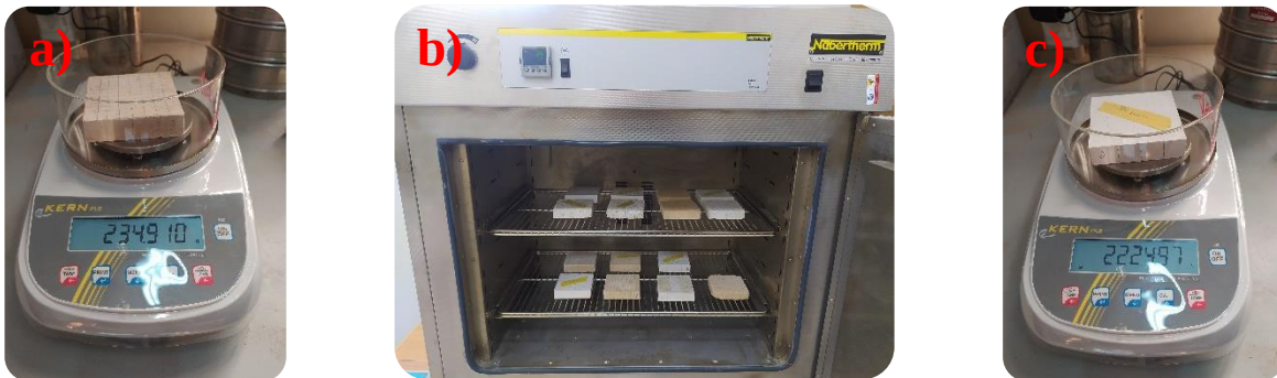
Figure III.19. Moisture Content Test: a) Specimen Weight before Drying, b) Drying Specimens in a Dryer, and c) Specimen Weight after Drying.
