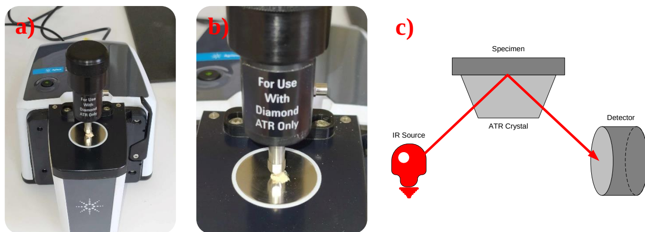
Figure III.23. Fourier Transform Infrared Spectroscopy (FT-IR) Test: a) Agilent Cary 630 Fourier-Transform Infrared (FT-IR) Device, b) The Specimen in an ATR crystal, and c) The FTIR Spectroscopy for Specimen Analysis.
