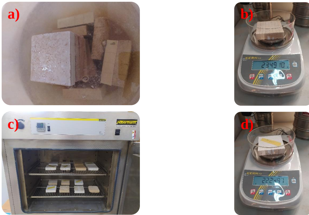
Figure III.17. Water Absorption Test: a) The Immersion of the Specimen, b) Weighing the Specimen after Immersion, c) Drying the Specimen, and d) Weighing the Specimen after Drying in the Dryer.
