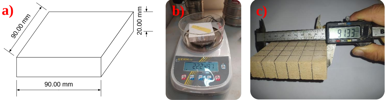
Figure III.16. Bulk Density Test: a) The Specimen Size, b) Weigh the Specimen, and c) The Specimen Measurements.
