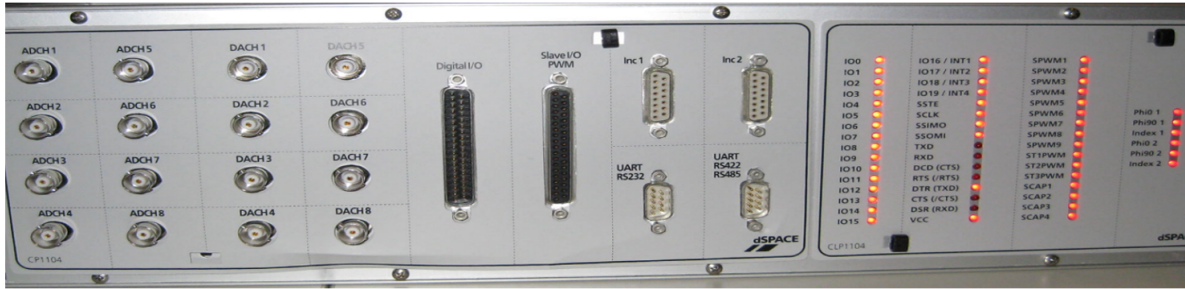
Figure 5.2: Connector panel of the dSPACE CLP1104 used for experiments.
